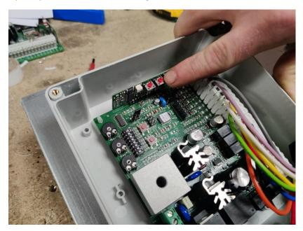
On the raised section, push and release the small red button closest to the cable connections, highlighted in this picture. The LED to the left of it will start to flash.
