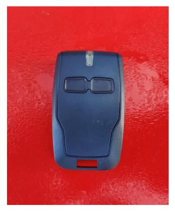
Take your new fob. Depress and hold both buttons down until a steady light is shown on the control board and the fob. Release both buttons and then push and release the button to which you want to pair the barrier.
